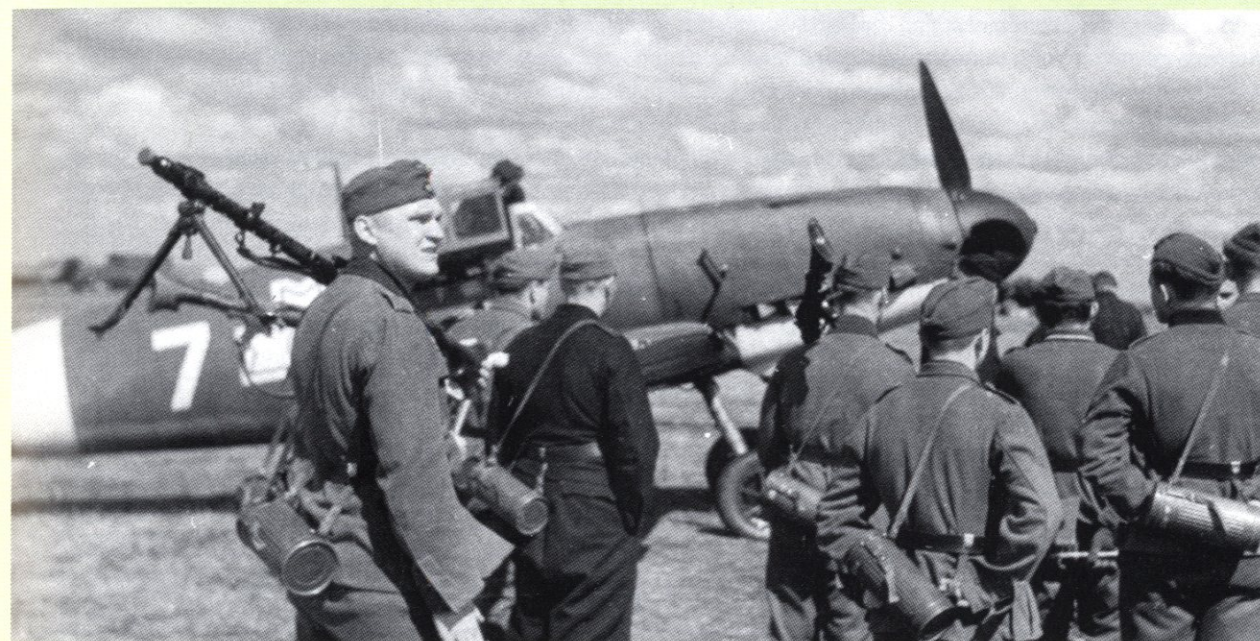
BELOW: German soldiers familiarising themselves with Rumanian aircraft at Dnepropetrovsk airfield. Parked in the background is a Bf 109 G-2 coded 'White 7'. Note that the undercarriage fairings on this aircraft have been removed.
