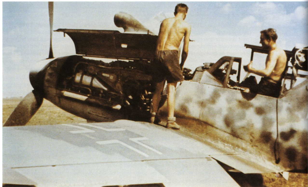
ABOVE AND RIGHT: 'White 10', a Bf 109 G-6 of I./JG 52 at Kharkov-Rogan, a major air base in Southern Russia, in the summer of 1943. Particularly well-shown in these views is the nature of the fuselage camouflage comprising light mottles of RLM 02 over RLM 76, followed by heavier mottles of the darker greys RLM 74 and 75.
