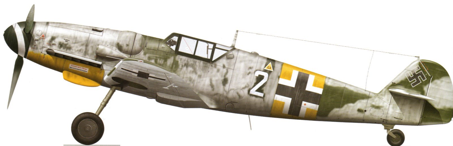
Messerschmitt Bf 109 G-6 'White 2', W.Nr. 412605, of IV./JG 54, Siverskaya, Winter of 1943/44 This aircraft had a weathered temporary white finish, beneath which were JG 54's characteristic dark greens although much of the canopy framing remained in the original 74 and 75 colours. No loop antenna was fitted to the baseplate situated on the fuselage just forward of the fuel filler point, and the radio mast was the shortened type. The undercarriage fairings on this machine had been removed.
