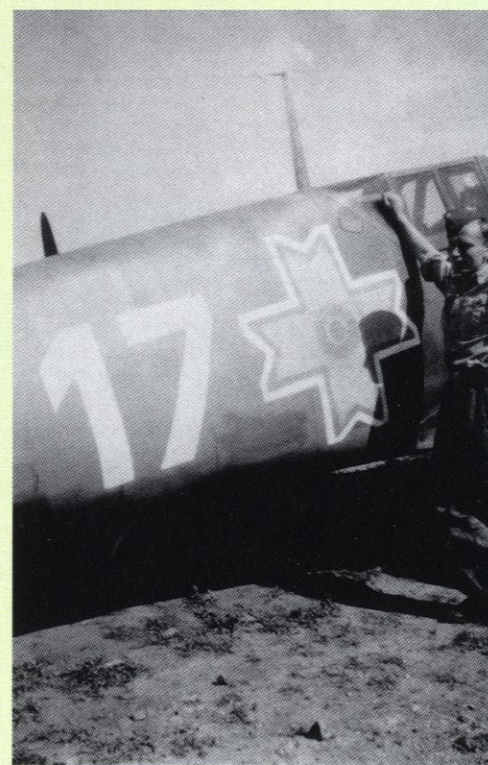
LEFT: From his position on the starboard wing, a member of the ground staff guides a Rumanian Bf 109 G-4 pilot over the airfield. This photograph, probably taken in the Ukraine in the summer of 1943, shows the dark green uppersurface camouflage and the hard demarcation line running from the leading edge of the tailplane to the training edge of the mainplane.
