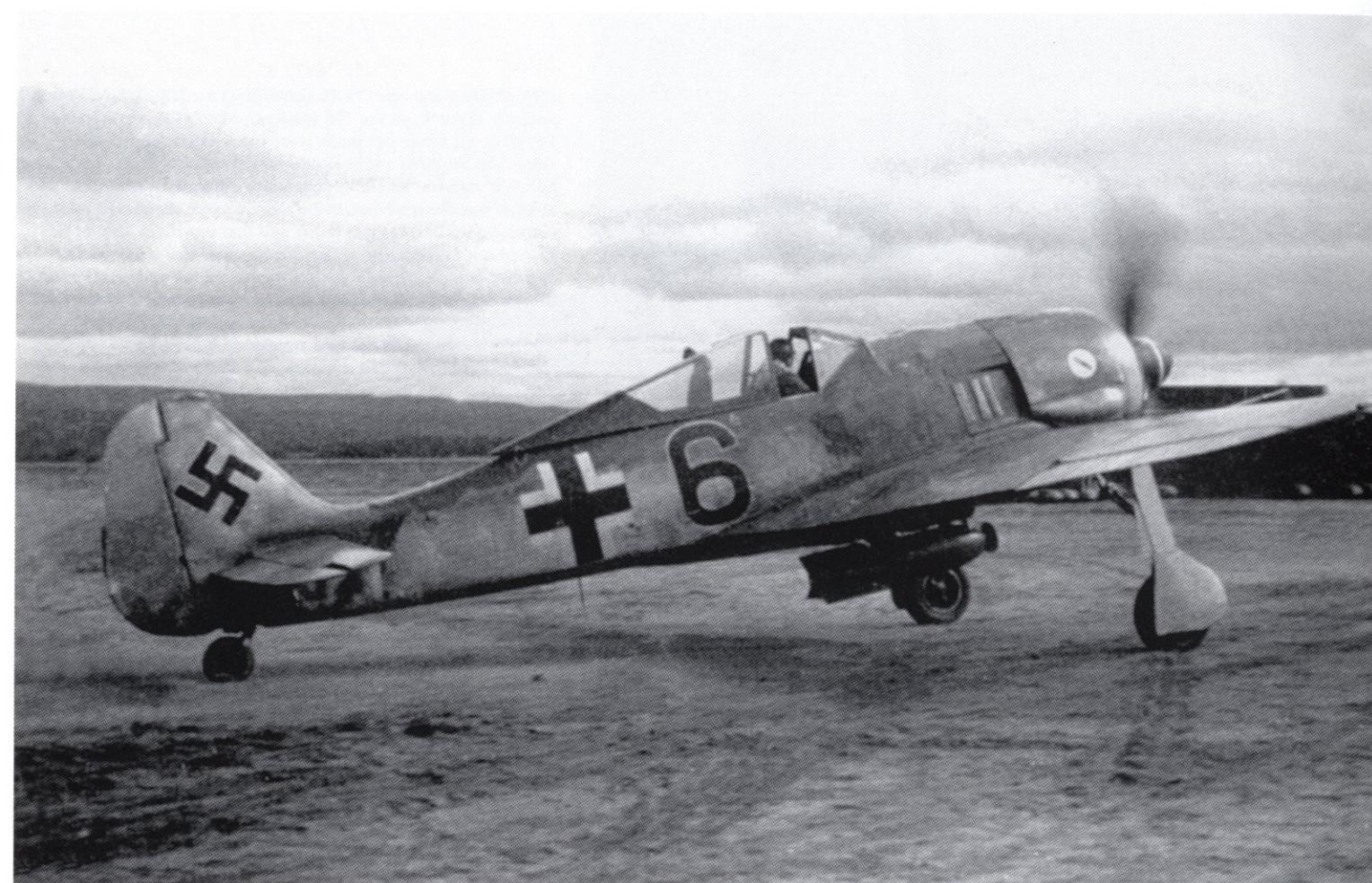
ABOVE: The oversize 'Black 6' on the fuselage of this Fw 190 A-3 of 14.(Jabo)/JG 5 taxiing with an SC 250 bomb is typical of this Staffel's aircraft. Note that as frequently observed on older models of the Fw 190 retained in service, this aircraft has been modified with the later pattern exhausts as fitted to the A-5. The circular plate on the front of the bomb was intended to ensure that the blast effect was maximised by detonating the bomb above ground.
