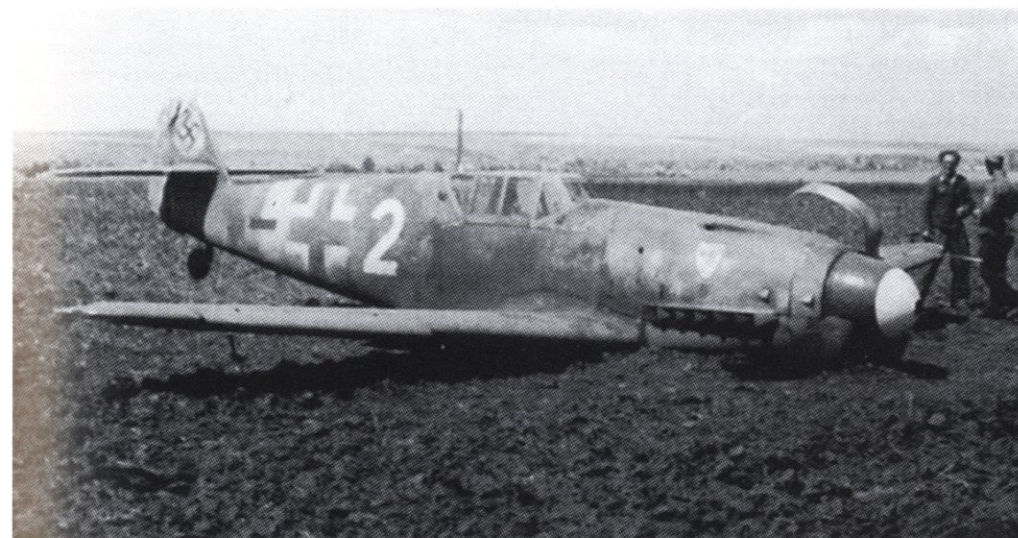
LEFT AND BELOW: This Bf 109G-2, 'White 2', belonged to 4./JG 3 and is pictured after making an emergency landing in February 1943. As may be seen here, it was usual practice with II./JG 3 at this time to show the Gruppe bar in black, regardless of the Staffel colour. The aircraft was camouflaged in an RLM 74/75/76 scheme with the fuselage sides being particularly densely mottled so that little of the RLM 76 was visible. In addition, the starboard side shows a large, dark stain, but as this is not present on the port side, it is thought that instead of carbon deposit from the exhaust, this may be oil and might possibly indicate the cause of the crash-landing. There is also some evidence, especially in the port view, that the machine received some unit-level modifications to the scheme. This is particularly noticeable under the cockpit, where there is a patch of an unusually dark colour, while the areas around the swastika and on the rudder appear to have been lightened with sprayed areas of RLM 76.
