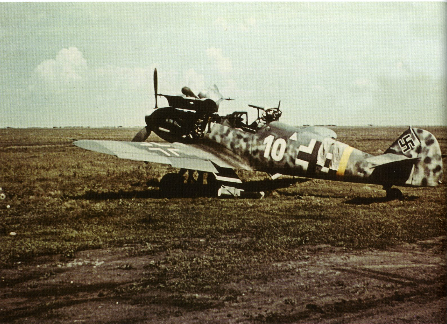
ABOVE AND RIGHT: 'White 10', a Bf 109 G-6 of I./JG 52 at Kharkov-Rogan, a major air base in Southern Russia, in the summer of 1943. Particularly well-shown in these views is the nature of the fuselage camouflage comprising light mottles of RLM 02 over RLM 76, followed by heavier mottles of the darker greys RLM 74 and 75.
