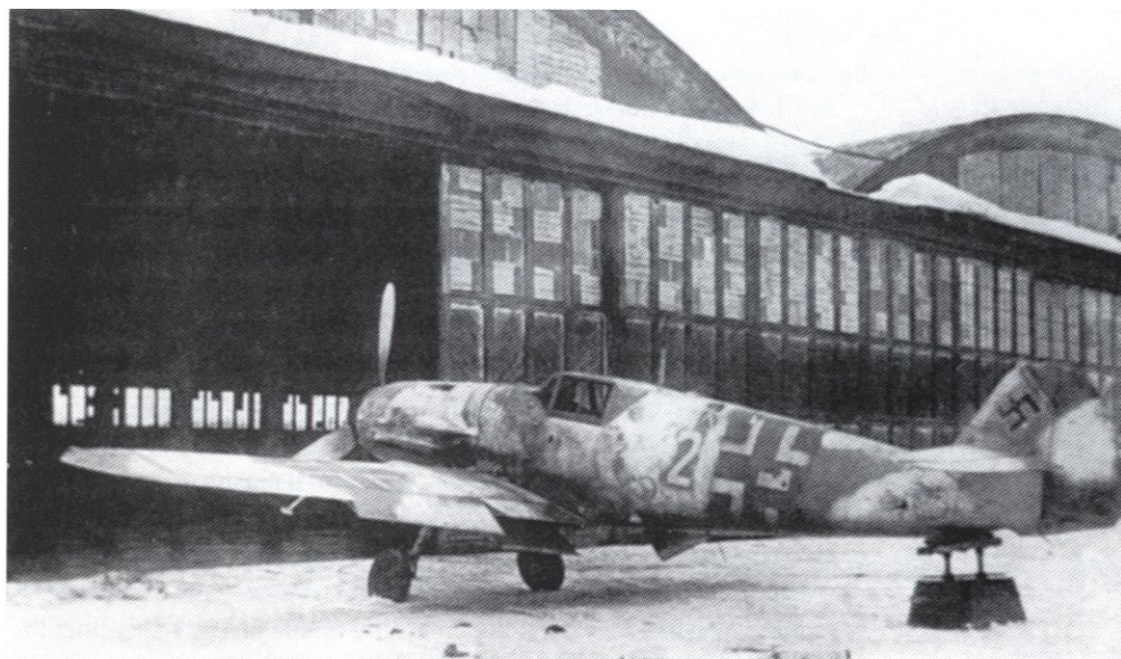
Messerschmitt Bf 109 G-6 'White 2', W.Nr. 412605, of IV./JG 54, Siverskaya, Winter of 1943/44 This aircraft had a weathered temporary white finish, beneath which were JG 54's characteristic dark greens although much of the canopy framing remained in the original 74 and 75 colours. No loop antenna was fitted to the baseplate situated on the fuselage just forward of the fuel filler point, and the radio mast was the shortened type. The undercarriage fairings on this machine had been removed.
