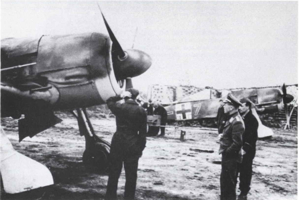
ABOVE AND RIGHT: Two more views of Lt. Emil Lang's 'Black 7' with (RIGHT), Oblt. Max Stotz discussing his 'Black 5' with technical personnel in the foreground. Like 'Black 5', 'Black 7' retained its inboard undercarriage doors and both aircraft have outboard wing armament. In the view (ABOVE), the wing in the foreground provides some indication of the extent of sand colouring and shows that the Balkenkreuze were the outline type.
