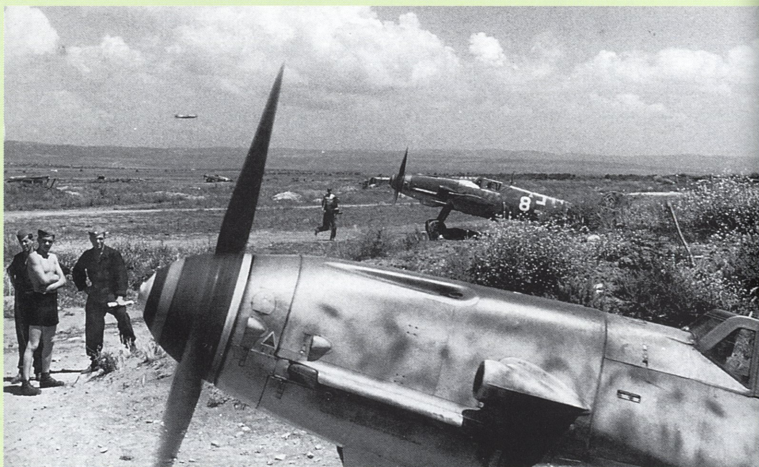
BELOW: Another scene at Anapa in the summer of 1943 showing aircraft of 13.(Slowak)/JG 52 preparing for a mission. Note the two groups of four holes on the cowling of the machine in the foreground. These were the mounting holes which, on tropical versions of the Bf 109 G series, were for the brackets which held the air cleaner in place.)
