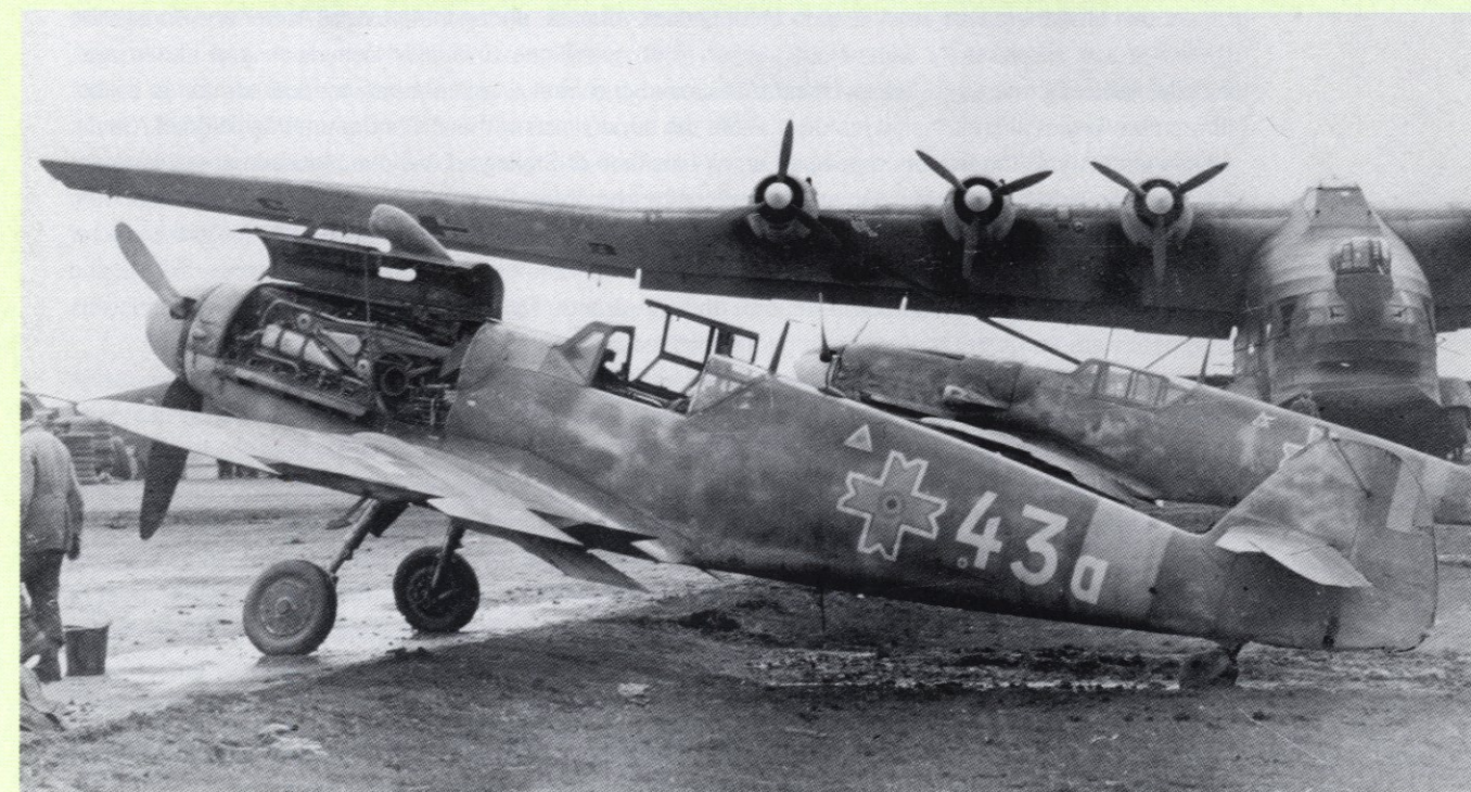
BELOW: A Rumanian Bf 109 G-2 'White 43a' with 'Yellow 1' behind and a Luftwaffe Me 323 'Gigant' in the background. Note again the absence of undercarriage fairings and the 'a' suffix to the aircraft number which indicates that this was a replacement machine for the original aircraft coded '43'. This photograph was probably taken in 1944.
